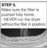
! Failure to clean the filter after EVERY drying cycle will affect the drying performance of your machine.
